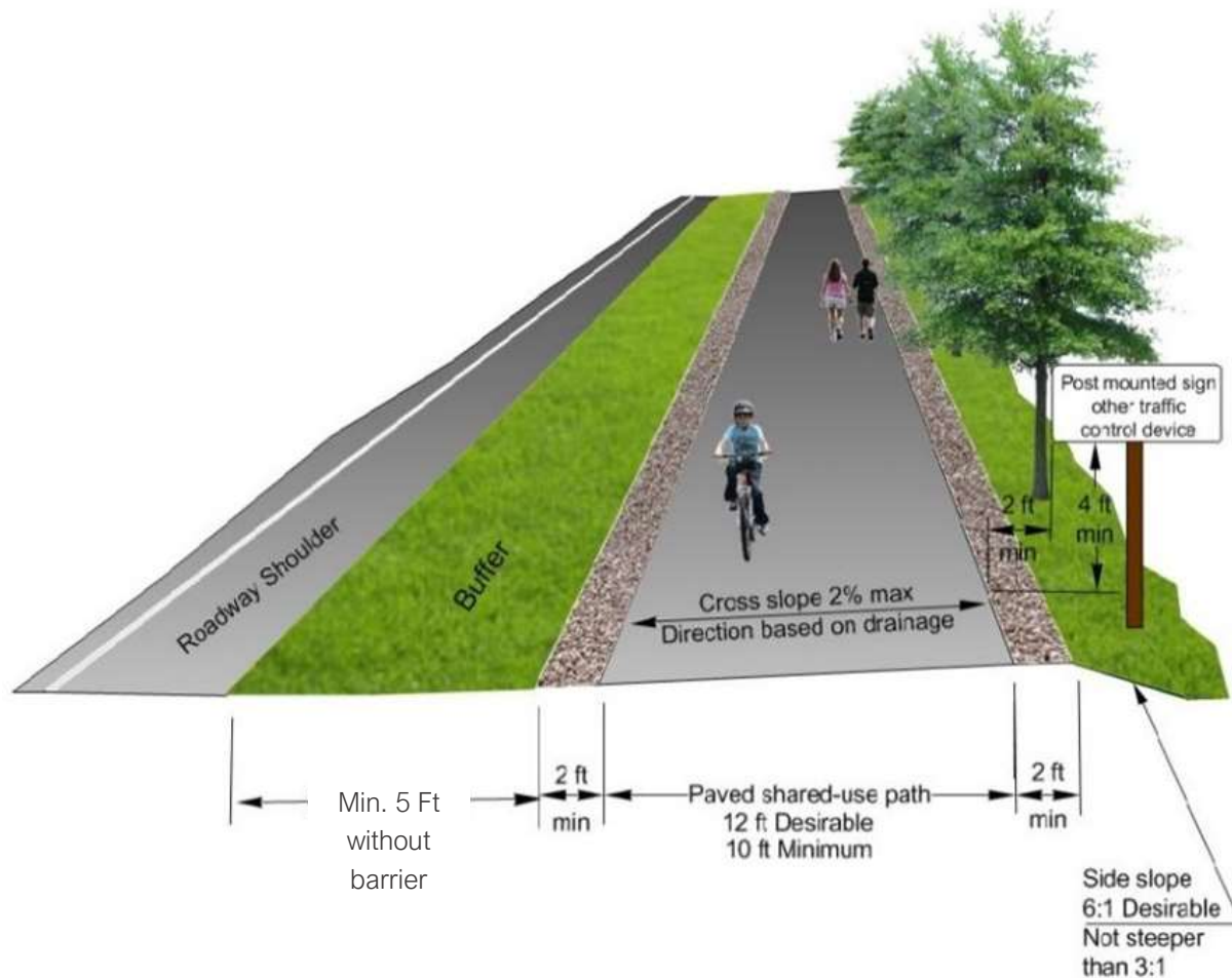
Figure 5: Two-Way Shared-Use Path Adjacent to Roadway (> 35mph) (Source: WSDOT Design Manual Exhibit 1515-5)
